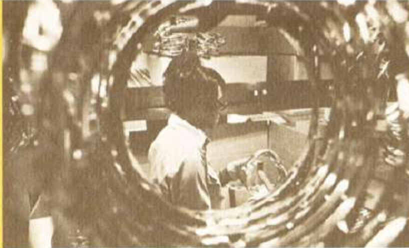
INSPECTION —A row of decorative headlamp parts frames an inspector as she examines the chromium finish of a bezel which fits around the Sealed Beam unit on a car.
